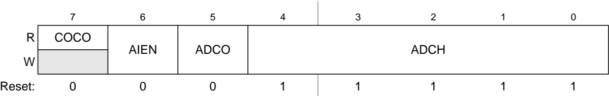
Figure 10-3. Status and Control Register (ADCSC1)
