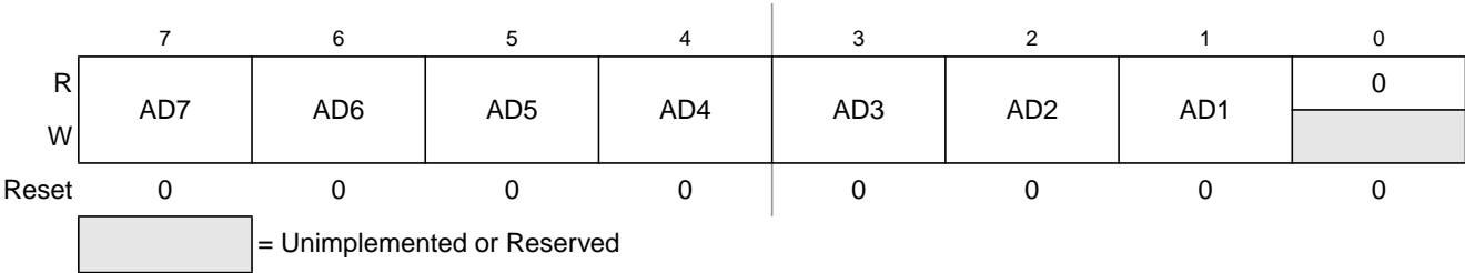
Figure 11-3. IIC Address Register (IICA)
