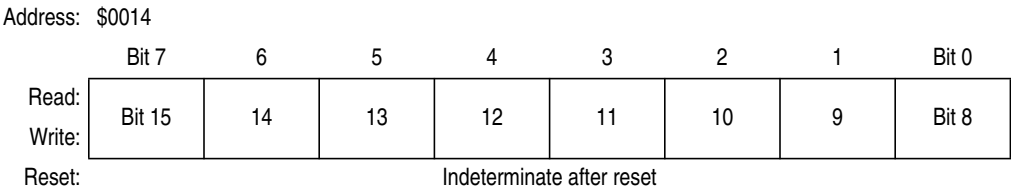
Figure 8-14. TIM Channel 1 Register High (TCH1H)
