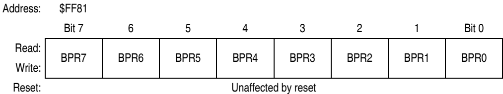
Figure 2-8. FLASH-2 Block Protect Register (FL2BPR)
