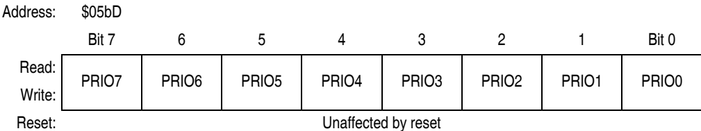
Figure 12-14. Transmit Buffer Priority Register (TBPR)
