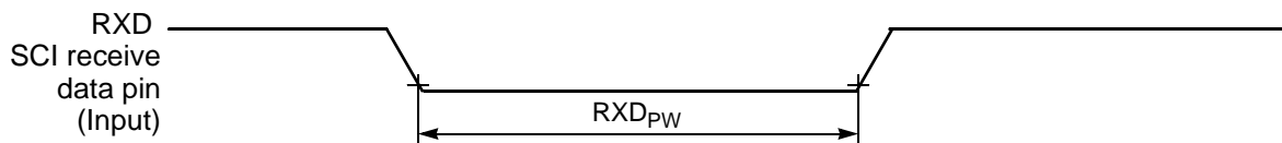
Figure 10-15 RXD Pulse Width
