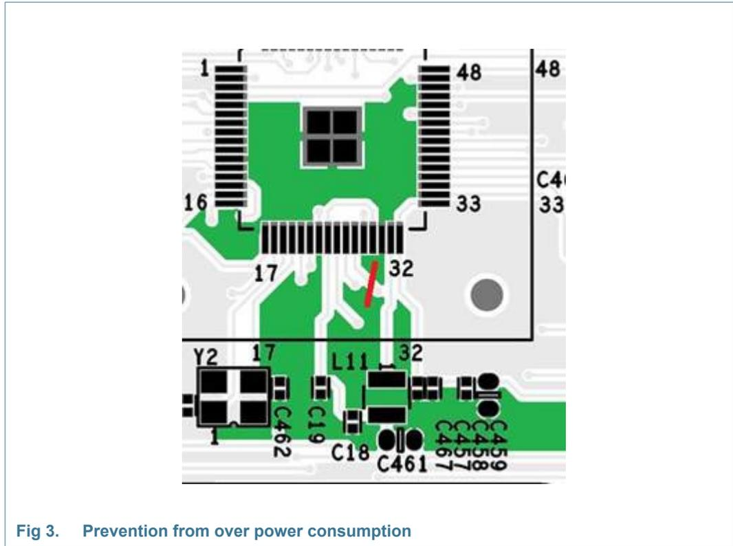
Fig 3. Prevention from over power consumption
