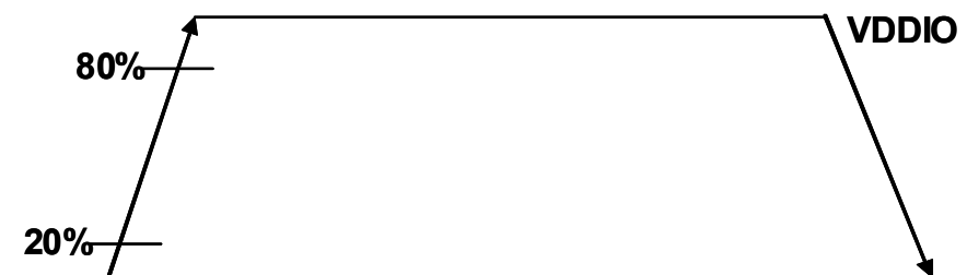
Figure 4. Output Pad Transition Waveform
