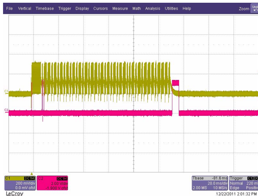
Figure 3-4. LF telegram used for MCU-direct mode example
