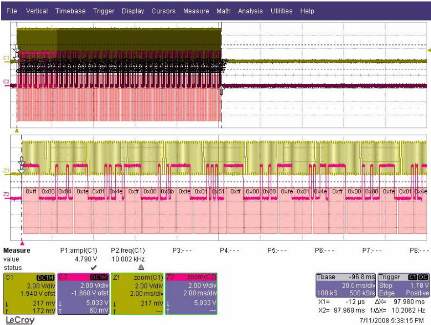
Figure 3-7. RF telegram received and decoded
