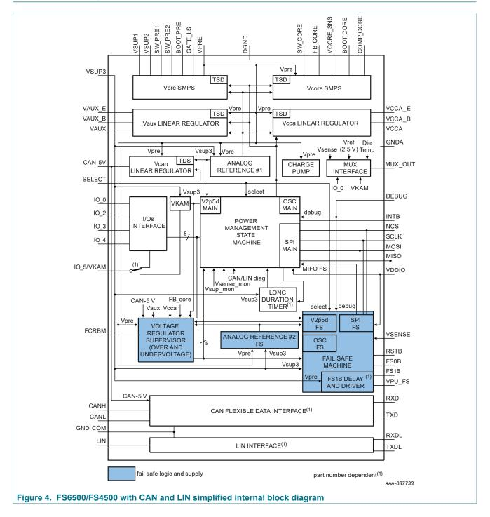
Safety power system basis chip with CAN FD and LIN transceivers
