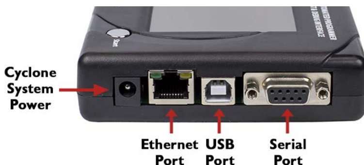
Figure 3-2: Cyclone FX Right Side View
