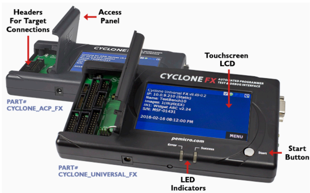
Figure 3-1: Cyclone FX Top View
