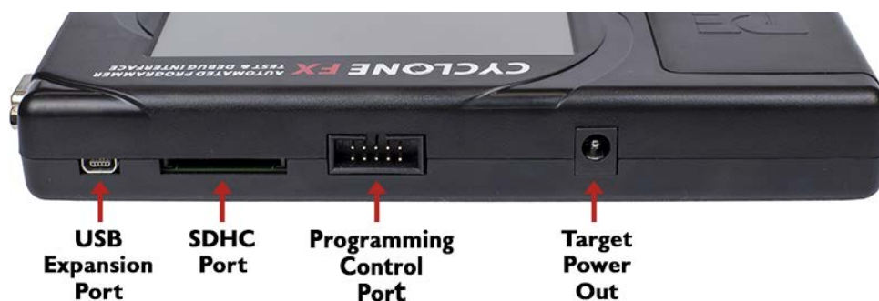
Figure 3-4: Cyclone FX Rear Side View
