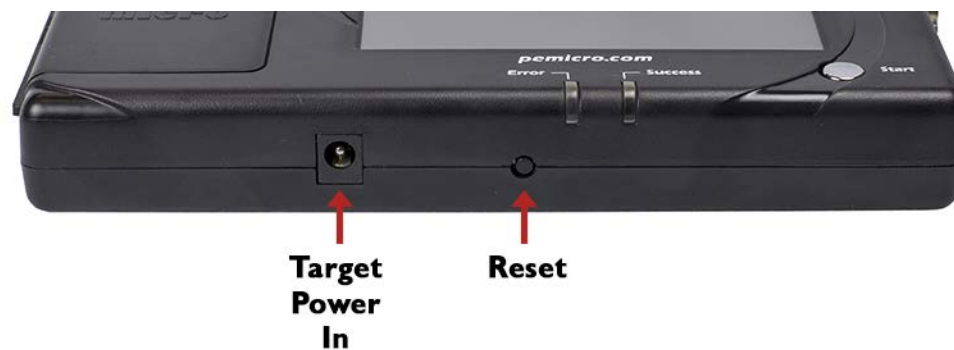
Figure 3-3: Cyclone FX Front Side View
