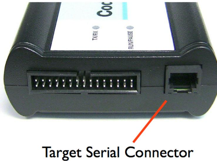
**Figure 14. CW TAP probe - target serial connector**
