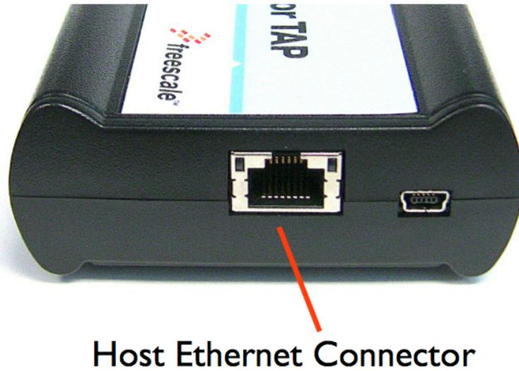
**Figure 3. CodeWarrior TAP probe with Ethernet connector**
