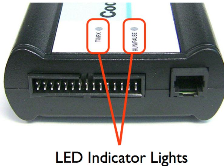
Figure 10. CW TAP probe - LED indicators
