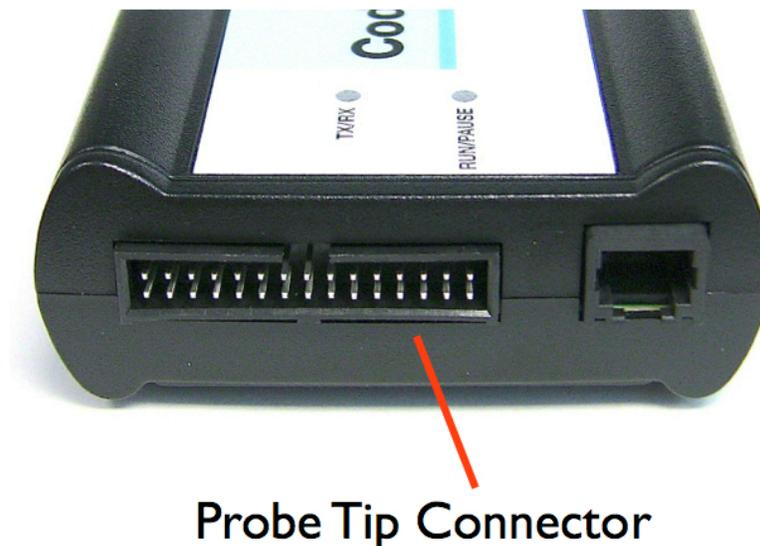
Figure 13. CW TAP probe - target side view
