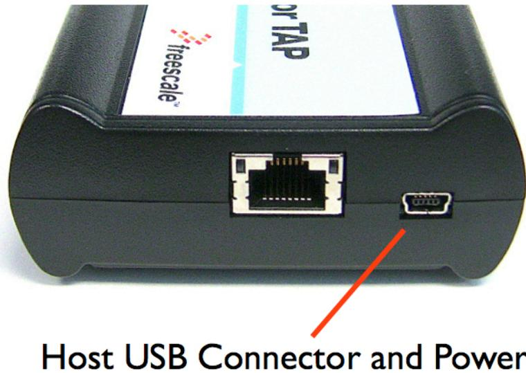
Figure 2. CodeWarrior TAP probe with USB connector
