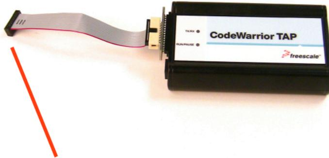
Connects to Target Debug Header
