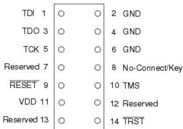
**Figure 19. CodeWarrior TAP probe OnCE connector pin assignments**
