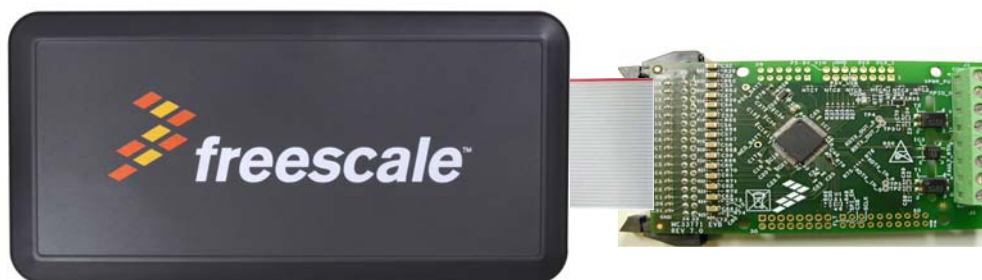
Figure 6. BATT-14AAAPACK Connection to KIT33771TPLEVB
