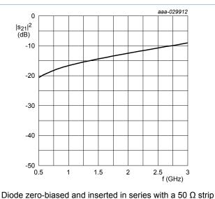
Diode zero-biased and inserted in series with a 50  $\Omega$  strip line circuit and biased via the analyzer T-network. T<sub>j</sub> = 25 °C; f = 1 MHz
