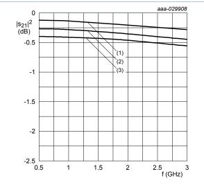
Diode inserted in series with a 50  $\Omega$  strip line circuit and biased via the analyzer T-network. T<sub>i</sub> = 25 °C; f = 1 MHz
