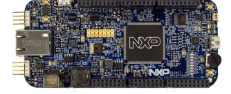
• Easy access to the MCU GPIO pins using available headers
