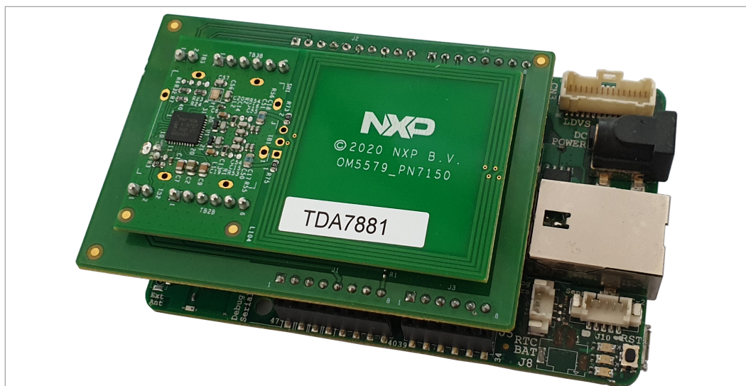
Figure 3. OM5579/PN7150ARD and UDOO Neo stacked together
