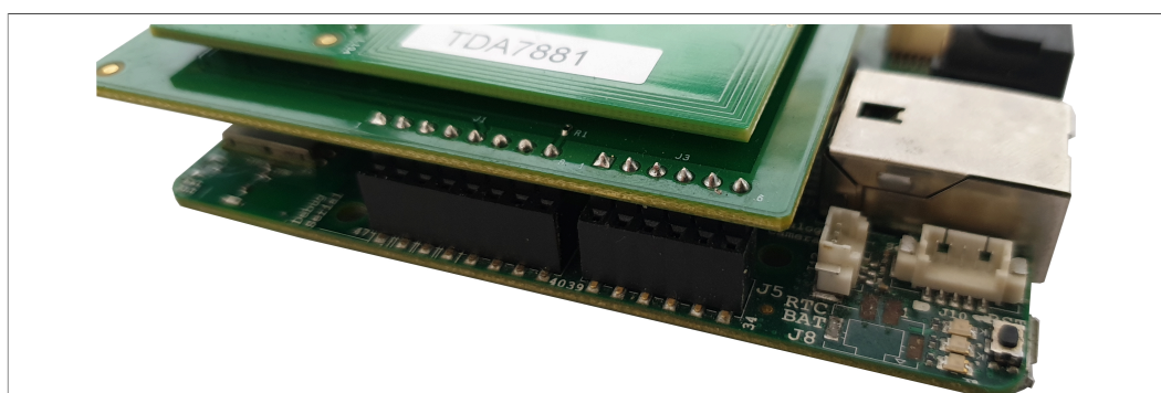
Figure 4. OM5579/PN7150ARD and UDOO Neo stacked together - zoom
