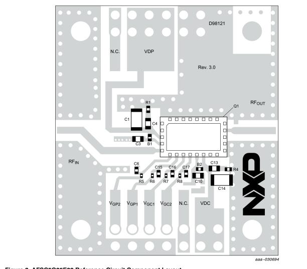
Figure 2. AFSC5G35E38 Reference Circuit Component Layout
