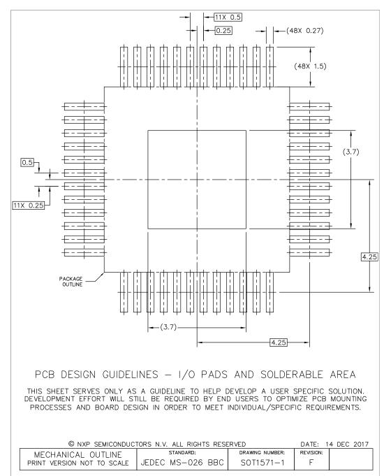
Figure 11. SOT1571-1 Rev. F - PCB design guidelines - I/O pads and solderable area
