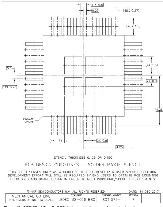
Figure 12. SOT1571-1 Rev. F - PCB design guidelines - solder paste stencil
