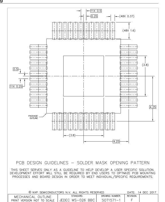
Figure 10. SOT1571-1 Rev. F - PCB design guidelines - solder mask opening pattern
