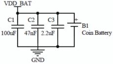
Figure 2. Capacitor at pin VDD\_BAT
