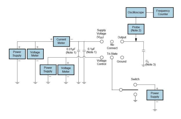
Note 1: An external 0.01µF ceramic bypass capacitor in parallel with a 0.1µF high frequency ceramic bypass capacitor close (less Than 2mm) to the package ground and supply voltage pin is required.
