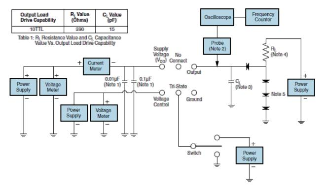
**Note 1:** An external 0.01µF ceramic bypass capacitor in parallel with a 0.1µF high frequency ceramic bypass capacitor close (less Than 2mm) to the package ground and supply voltage pin is required.
