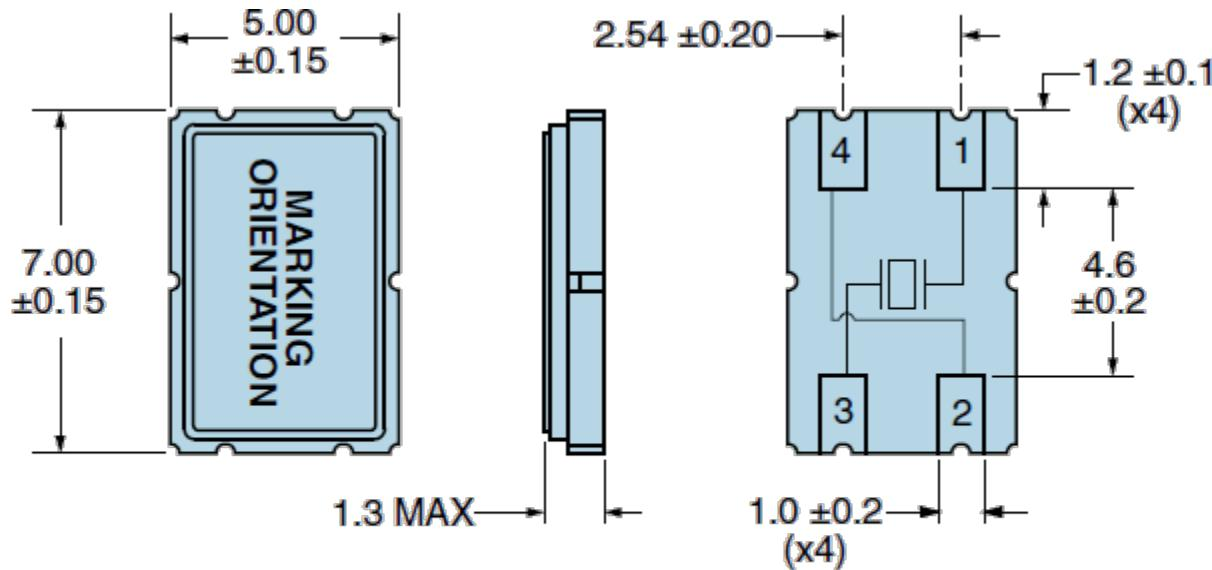
**Terminal Plating Thickness:** Gold (0.3 to 1.0 $\mu$ m). Nickel (1.27 to 8.89 $\mu$ m).
