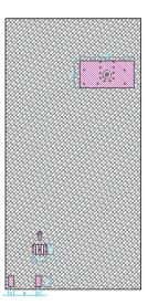
₩ Welding paint Bottom Layer ■ Bare copper area
