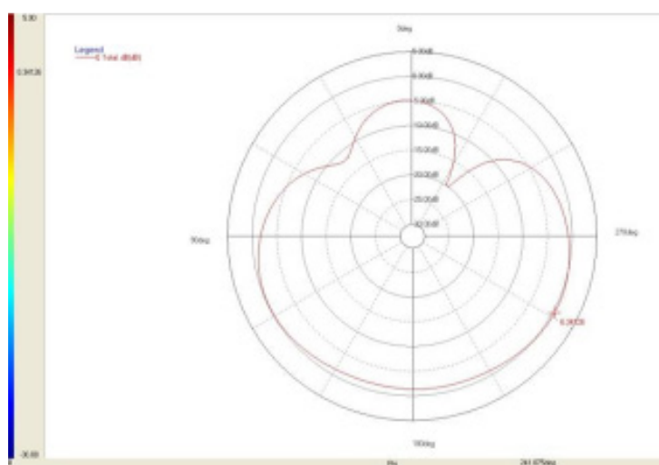
2D Radiation Pattern X-Y Plane 2450MHz
