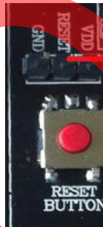
Figure 8: Jumper setting for high effective RESET
