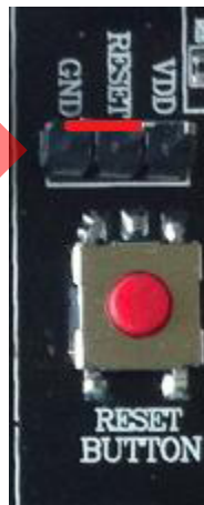
Figure 9: Jumper setting for low effective RESET
