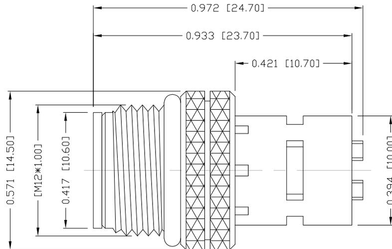
3 = BRASS/TIN (B/T) SHELL & BRASS/NICKEL NUT
