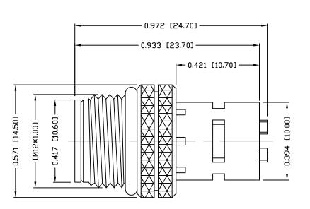
NΠΤΕ: MATERIAL HOUSING: PBT UL94V-0, BLACK CONTACT: BRASS NUT: BRASS □-RING: EPDM, BLACK SHELL: BRASS FINISH CONTACT: GOLD PLATED □VER 504" NICKEL NUT: NICKEL PLATED SHELL: BRIGHT TIN PLATED ELECTRICAL RATED CURRENT: 4A RATED VOLTAGE: 60V INSULATION RESISTANCE: 100 MOhms MIN. CONTACT RESISTANCE: 10 mOhms MAX. IP67 WATER PROOF: **ENVIRONMENT** -40°C TD +85°C OPERATION TEMPERATURE: MAX WIRE AWG: 22
