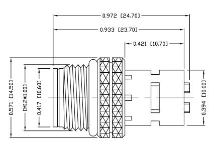
NΠΤΕ: MATERIAL HOUSING: PBT UL94V-0, BLACK CONTACT: BRASS NUT: BRASS EPDM, BLACK □-RING: SHELL: BRASS FINISH CONTACT: GOLD PLATED □VER 504" NICKEL NUT: NICKEL PLATED SHELL: BRIGHT TIN PLATED **ELECTRICAL** RATED CURRENT: 4A 250V RATED VOLTAGE: INSULATION RESISTANCE: 100 MOhms MIN. CONTACT RESISTANCE: 10 mOhms MAX. IP67 WATER PROOF: **ENVIRONMENT** OPERATION TEMPERATURE: -40°C TD +85°C 22 MAX WIRE AWG:
