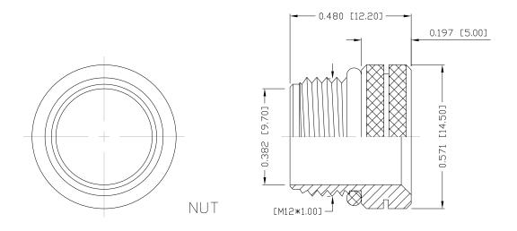
NOTE: MATERIAL HOUSING: PBT UL94V-0, BLACK BRASS CONTACT: NUT: BRASS D-RING: EPDM, BLACK FINISH CONTACT: GOLD PLATED OVER 504" NICKEL NICKEL PLATED NUT: 60ц" ТО 100ц" OVER ALL ELECTRICAL RATED CURRENT: 4Α 250V
