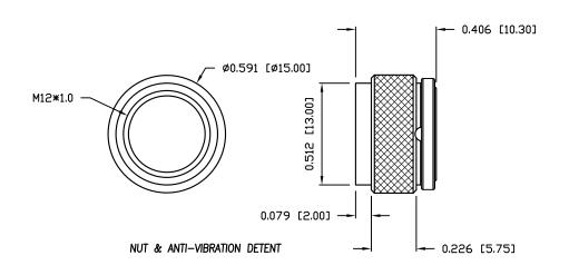
NΠΤF: MATERIAL HOUSING: PA66 UL94V-0, BLACK CONTACT: **BRASS** NUT: **BRASS** □-RING: EPDM, BLACK FINISH 10u" GOLD PLATED CONTACT: **NICKEL** NUT: ELECTRICAL RATED CURRENT: 4A 250V RATED VOLTAGE: INSULATOR RESISTANCE: 100 MOhms MIN.
