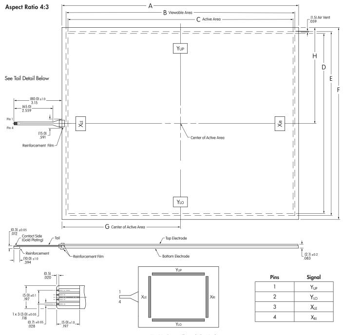
Yup, Ylo: Bottom Electrode Terminal Xle, XRI: Top Electrode Terminal
