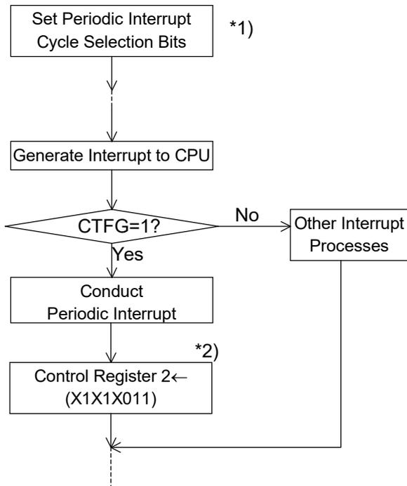
\*1) This step is intended to select the level mode as a waveform mode for the periodic interrupt function.
