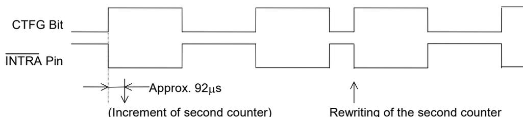
In the pulse mode, the increment of the second counter is delayed by approximately 92  $\mu$ s from the falling edge of clock pulses. Consequently, time readings immediately after the falling edge of clock pulses may appear to lag behind the time counts of the real-time clocks by approximately 1 second. Rewriting the second counter will reset the other time counters of less than 1 second, driving the INTRA pin low.
