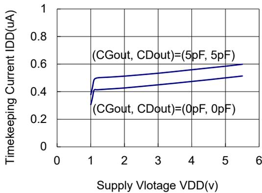
Time Keeping Current vs. Supply Voltage
