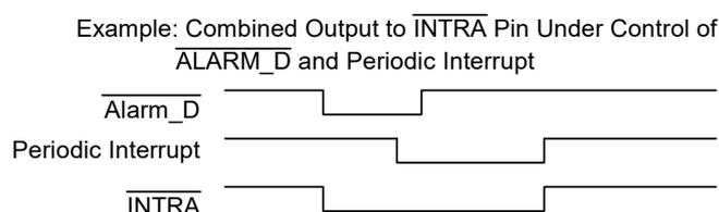
In this event, which type of interrupt signal is output from the  $\overline{\text{INTRA}}$  pin can be confirmed by reading the DAFG, and CTFG bit settings in the Control Register 2.
