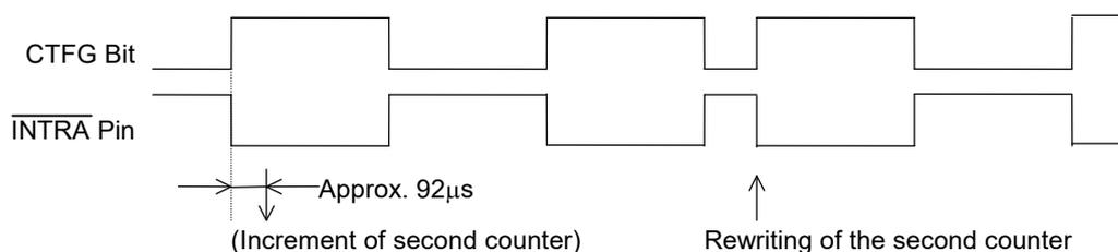
In the pulse mode, the increment of the second counter is delayed by approximately 92 μs from the falling edge of clock pulses. Consequently, time readings immediately after the falling edge of clock pulses may appear to lag behind the time counts of the real-time clocks by approximately 1 second. Rewriting the second counter will reset the other time counters of less than 1 second, driving the INTRA pin low.
