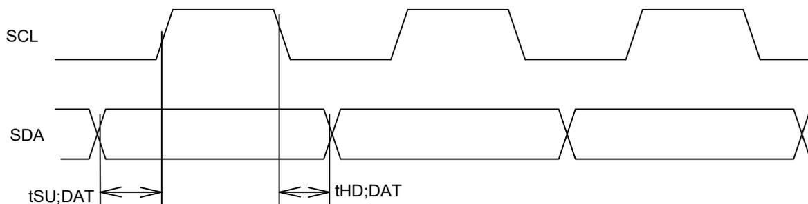
The SCL and SDA pins are at the “H” level when no data transmission is made. Changing the SDA from “H” to “L” when the SCL and the SDA are “H” activates the Start Condition and access is started. Changing the SDA from “L” to “H” when the SCL is “H” activates Stop Condition and accessing stopped. Generation of Start and Stop Conditions are always made by the master (see the figure below).
