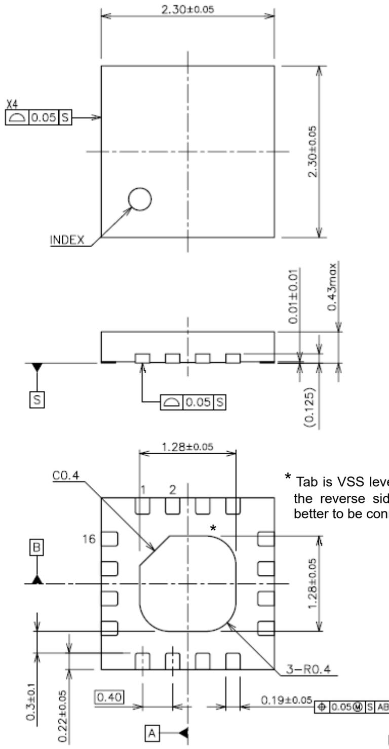
\* Tab is VSS level. (They are connected to the reverse side of this IC.) The tab is better to be connected to the VSS.
