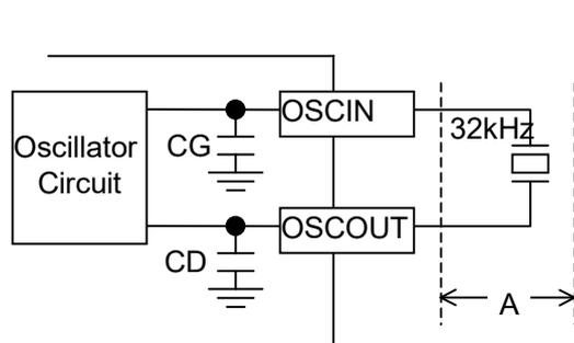
Typical externally-equipped element
