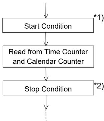
\*1) When reading to clock and calendar counters, do not insert Stop Condition until all times from second to year have been written to prevent error in writing time. (Detailed in "P.31 Data Transmission under Special Condition".
