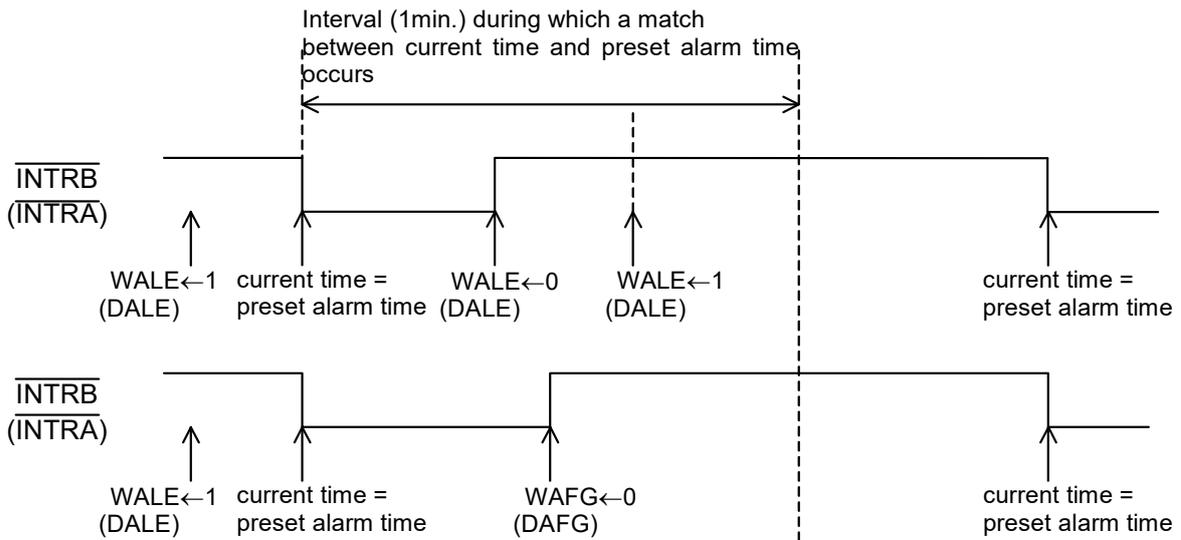
After setting WALE(DALW) to 0, Alarm registers is set to current time, and WALE(DALE) is set to 1,  $\overline{\text{INTRB}}$  or  $\overline{\text{INTRA}}$  will be not driven to "L" immediately,  $\overline{\text{INTRB}}$  or  $\overline{\text{INTRA}}$  will be driven to "L" at next alarm setting time.
