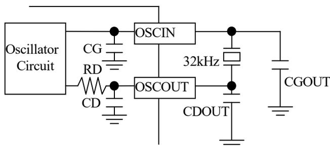
\*1) The CGOUT or/and CDOUT should have a capacitance ranging from 0 to 6 pF.
