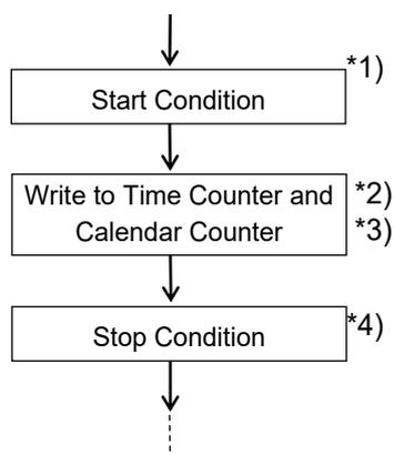
\*1) When writing to clock and calendar counters, do not insert Stop Condition until all times from second to year have been written to prevent error in writing time. (Detailed in "P.31 Data Transmission under Special Condition".
