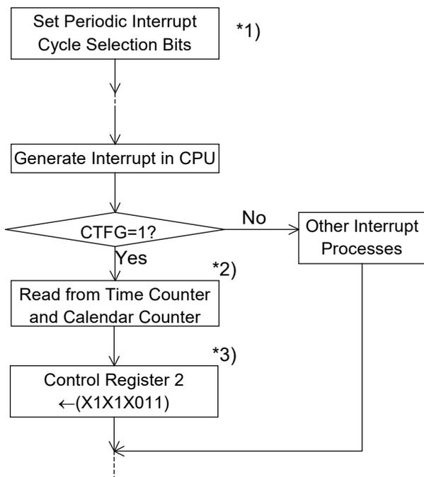
\*1) This step is intended to select the level mode as a waveform mode for the periodic interrupt function.
