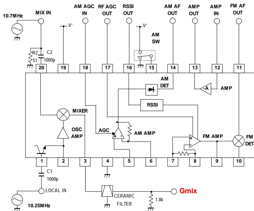
■ TERMINAL FUNCTION (Ta=25°C , V<sup>+</sup>=2.7V , circuit 1)
