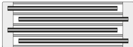
Extended double side metallized carrier film design
