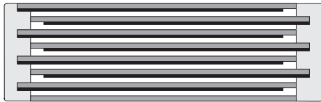
Extended metallized film design
