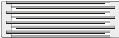
Extended metallized film design
