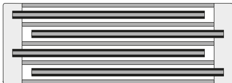
Extended double side metallized carrier film design
