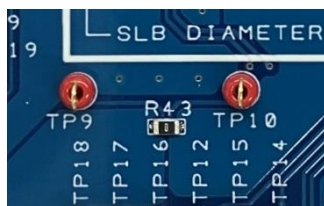
Fig. 4-3-6b Current monitoring resistor and test pins
