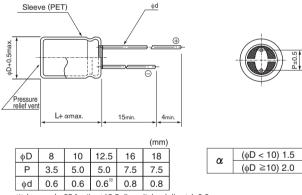
In case L>25 for the φ12.5 dia unit, lead dia φd=0.8
