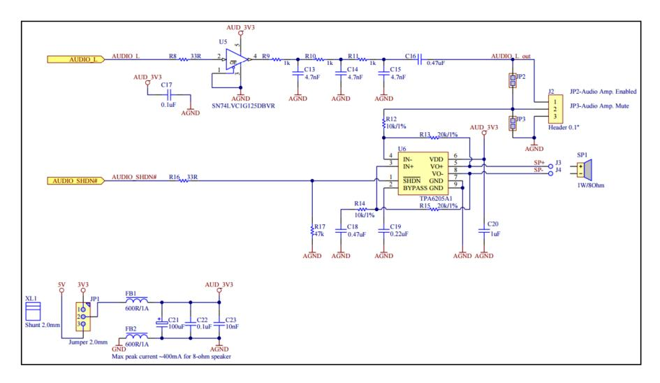
This is a reference schematic from FTDI, which can be used to successfully filter and amplify the audio signals coming from the NHD EVE TFT Module.
