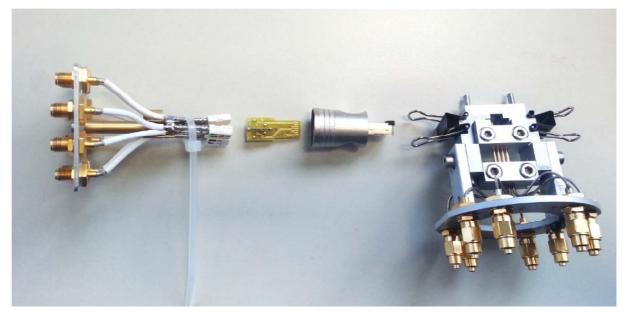
Exploded view of the test setup. The connector body was opened to access the RJ45 connector interface. RG 188 coaxial cables connected the printed circuit board to the network analyzer. A standard compliant direct probe fixture by Telegärtner terminated the test setup.
