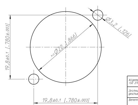
min. Einbauabstand min assembling distance
