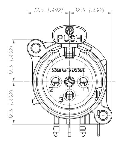
min. Einbauabstand min assembling distance
