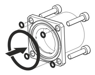
**NOTE** - IP68 Sealing Kits (5 chassis connectors can be sealed with one KIT)
