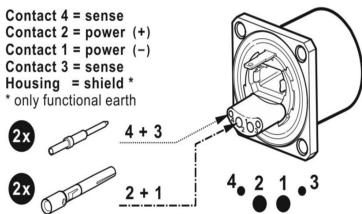
**POS-XP-SENSE** - The POS-XP-SENSE Crimp die is used for the assembly of the sense cooper pins.
