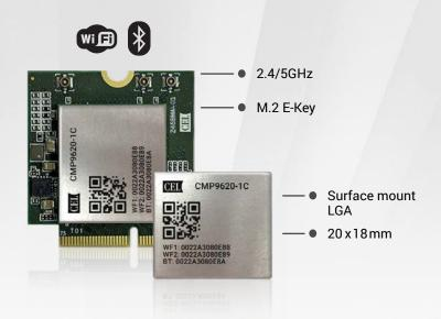
New wireless deployments demand more data throughput and more efficient network utilization. CEL designed the CMP9620 to deliver both, While offering out-of-the-box integration into NXP's I.MX8 ecosystem. Simultaneous Dual-Band operation, combined with concurrent Bluetooth and the latest Bluetooth features, deliver the connectivity demanded by Edge Gateways, HUBS and other High-Banwidth applications.
