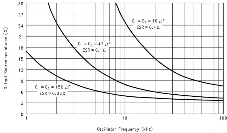
**FIGURE 4. Output Source Resistance vs Oscillator Frequency**
