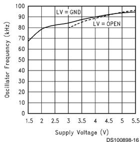
Oscillator Frequency vs Supply Voltage (FC = Open)
