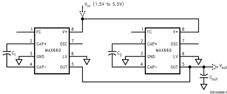
**FIGURE 5. Lowering Output Resistance by Paralleling Devices**
