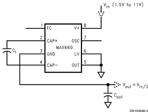
FIGURE 3. Splitting V<sub>IN</sub> in Half
