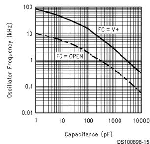
Oscillator Frequency Supply Voltage (FC = V+)
