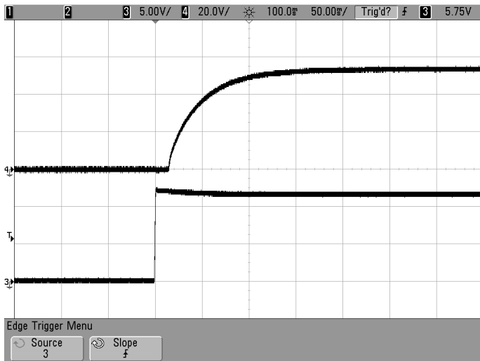
Vin Startup Delay, Vin = 12V, Iout = 4.44A, Channel #3 = 5V/div - Vin, Channel #4 = 20V/div - Vout, Ta = 25°C, Load = 1620µF
