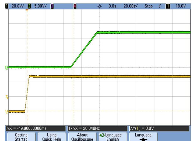
Figure 11. Vin Start-up Delay (CH2: Vout, CH1: Vin) (Vin=48V, Iout=50A, Cload=330μF, Ta=+25°C, 20mS/div)
