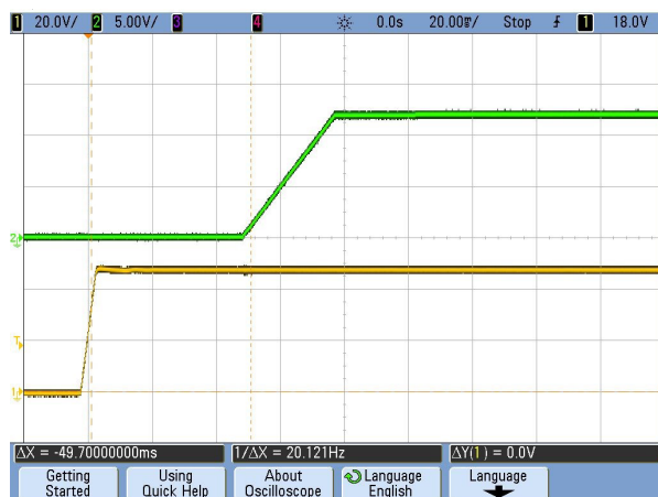
Figure 10. Vin Start-up Delay (CH2: Vout, CH1: Vin) (Vin=48V, Iout=0A, Cload=330μF, Ta=+25°C, 20mS/div)
