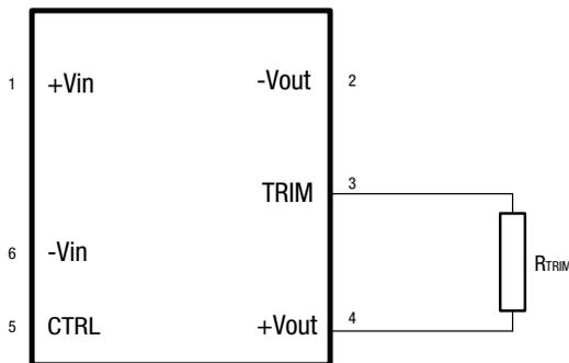
$$3.3V_{out} R_{TRIM} = \frac{18.64k \times V_{out} - 52.3k}{3.32 - V_{out}} \quad 5V_{in} 12V_{out} R_{TRIM} = \frac{30.4k \times V_{out} - 194.723k}{12.0744 - V_{out}}$$
