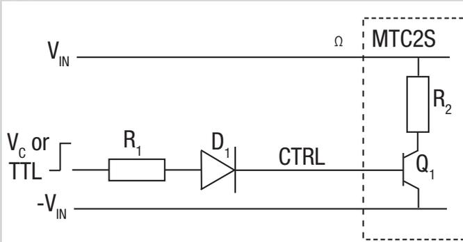
$D_1$  (e.g. 1N4001) is necessary for correct operation of the MTC2 when the control signal is LOW. The recommended drive current  $I_b$  to shut down the MTC2 is 6mA to 15mA. The value of  $R_1$  can be derived as follows:
