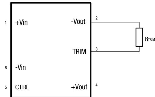
$$3.3V_{out} R_{TRIM} = \frac{14k \times V_{out} - 52.3k}{3.32 - V_{out}} \quad 5V_{in} 12V_{out} R_{TRIM} = \frac{12.4k \times V_{out} - 194.723k}{12.0744 - V_{out}}$$
