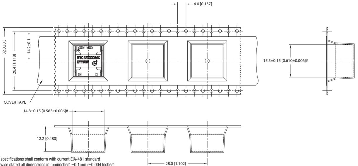
Tape & Reel specifications shall conform with current EIA-481 standard
