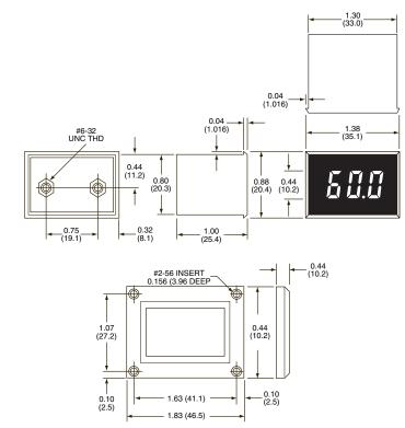
Dimensions in inches (millimeters) Tolerances: 2 PL Dec ±0.02 (±0.51) 3 PL Dec ±0.010 (±0.254) Recommended panel cutout dimensions: 1.336 (33.93)W × 0.838 (21.29)H Internal corner radii 0.032 (0.81) Max.
