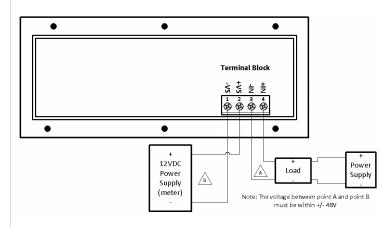
In this example, the load connects to terminals 3 and 4, where terminal 3 is the negative input terminal (-IN) and terminal 4 is the positive input terminal (+IN). The 12V power supply connects to terminals 1 and 2, where terminal 1 is the negative power supply terminal (-VS) and terminal 2 is the positive power supply terminal (+VS).
