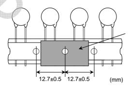
Splicing tape(Base and adhesive tapes aare inserted in a splicing tape.)
