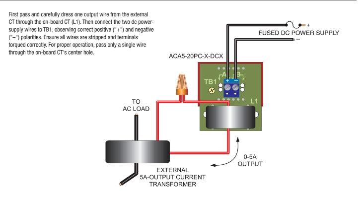
Figure 4. ACA5-20PC DC-Powered Models
