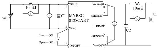
C1: Low Impedance Electrolytic Capacitor 100µF
